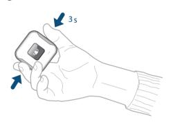
Press the side buttons for 3 seconds to send an alarm. An alarm icon will be displayed on the devices' screen and an SOS message will be sent together with the localisation information to the numbers that have been configured as emergency contacts and/or a call centre if configured (see the ALARMS section on the other side of this manual).
