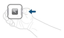
Press the right side button to pick up an incoming call. All incoming calls are managed hands free. If the QTrak GPS-023/GPS-024 device is handling an alarm situation, the incoming call will be picked up automatically.
