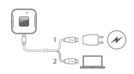
Connect the USB cable to the AC current adaptor (1) or to the USB port of your PC (2). Connect the other end to the micro USB port of your QTrak GPS-023/GPS-024 device that can be found under the USB cover.
