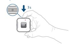
To switch on the QTrak GPS-023/GPS-024, press the On/Off button continuously for 3 seconds until the device's LED lights up and the welcome screen is displayed.
